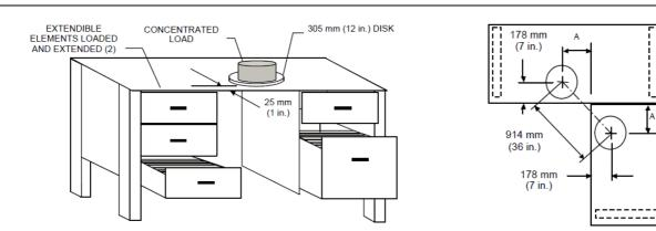
Height from the floor: 753 mm Distance of the load disk (305 mm diameter) center from the table edge: 178 mm Length of sample: 1575 mm
